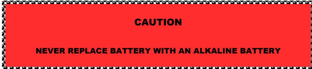
This unit has a rechargeable Lithium Ion battery and should only be charged with the supplied charger. Should the battery ever need replacing please contact Capri Electronics, LLC for the correct battery with the proper insulating padding.
