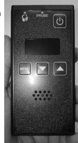
Use the TD-62 to perform a professional RF sweep of your premises. Similar in operation to a Geiger counter, the sensitive antenna system can be used to probe all areas of a room. As the antenna approaches the hidden transmitter, the audible tone clicks faster and faster while the signal strength is displayed in a bar graph on the units LCD screen.
